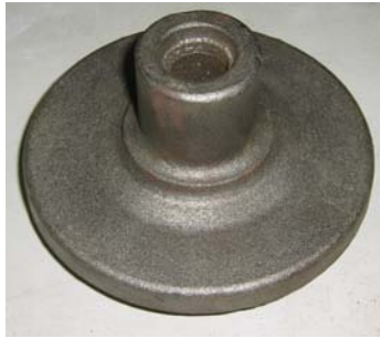
(a) Forged hub with a crack running from the flat surface to the radius
