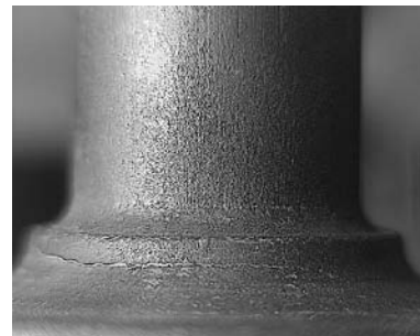
(b) Crack in the fillet radius
